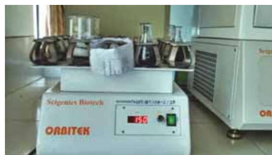
Figure 3. Foundry effluent being rotated at 150 rpm in mechanical shaker
