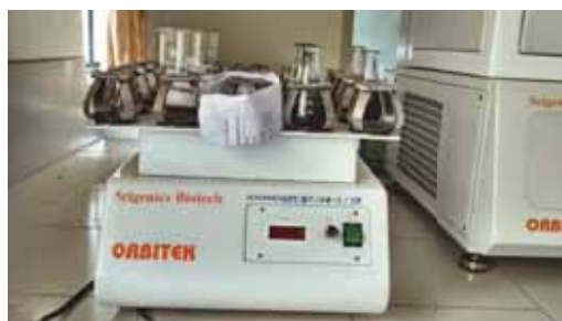
Figure 4: Foundry effluent being rotated at different speed
