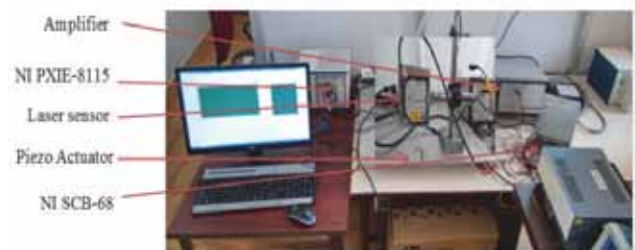
Fig. 8 Experimental setup to obtain displacement data for applied voltage for 1Hz frequency
