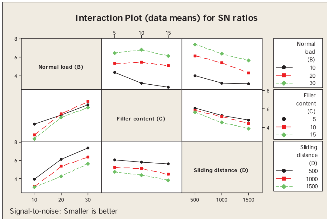
Fig. 3 Interaction graph between B, C and D for friction coefficient (S/N Ratio).
